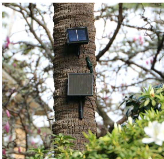
Two solar panels, feeding a string of fairy lights each set high on the trunk of a palm tree to catch the sun.
